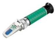
A simple density meter confirms salinity and verifies the ship carried out deep ocean exchange
